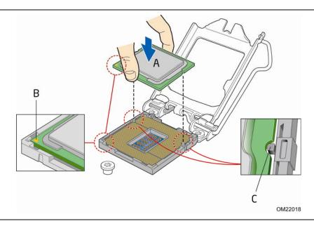
**Figure 10. Install the Processor**
